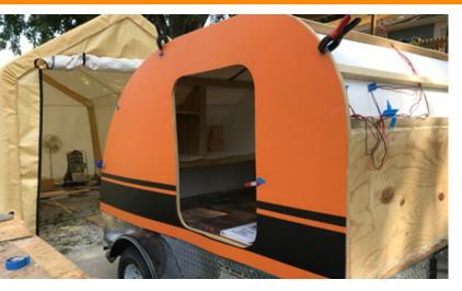
The exterior was skinned with FRP turned to the backside. I used Sherwin William exterior paint and then coated it with Flex Seal rubber coating. The roof is also FRP and sealed with Flex Seal tape. I went this route because I tend to change my mind often, and I knew I would want to change the designs on the sides.
