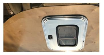
While the plans gave step by step instructions for doors, the awesome guys at Purdy Teardrops (recently purchased by Teardrops NW) sent two silver HEHR prefab doors. I love the built in sliding windows in these doors and the fact they are waterproof. Cutting the holes proved very easy and the install went quick, once I tossed the hand sander and started using the electric palm sander. While, the under-floor storage make the doors sit higher than most teardrops, it has not
