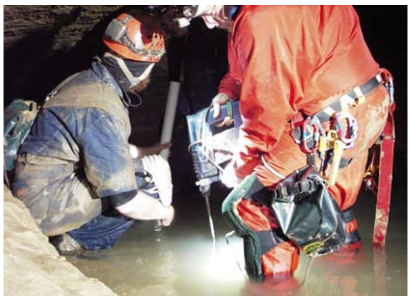
Drilling a hole in the bottom of the stream with a hammer drill. We anchored a stilling well to the stream bottom to protect a data logger. The data logger measures water depth and temperature.
