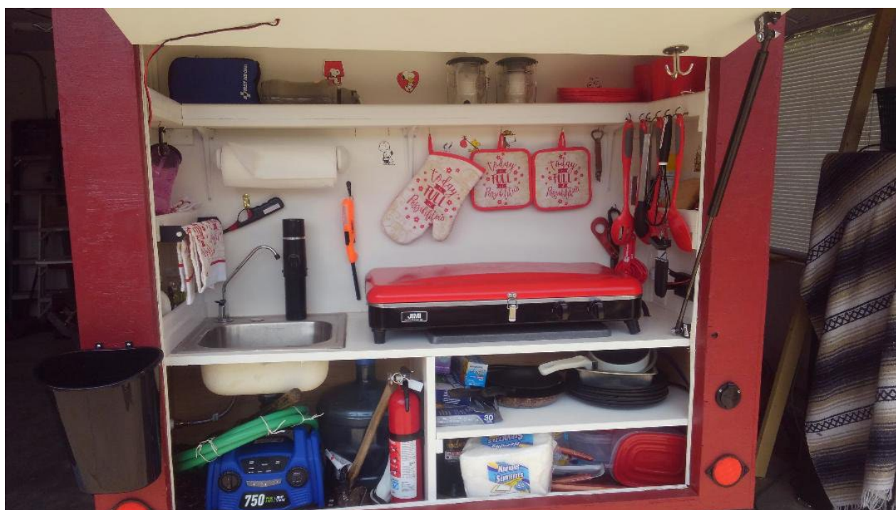
Above: The completed galley with the power pack under the sink. The shelves and hooks were added for additional storage.
